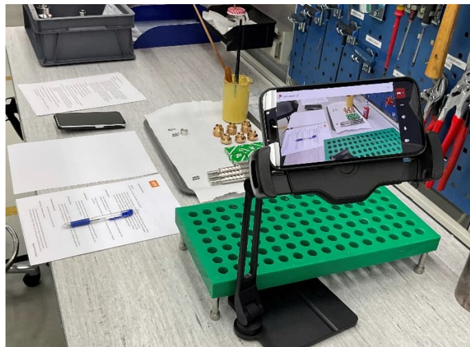
Figure 3. Test set-up. The test was recorded with a mobile phone in a manner that respected the anonymity of the participants. The AI assistant was accessed using the other smartphone on the desk.
